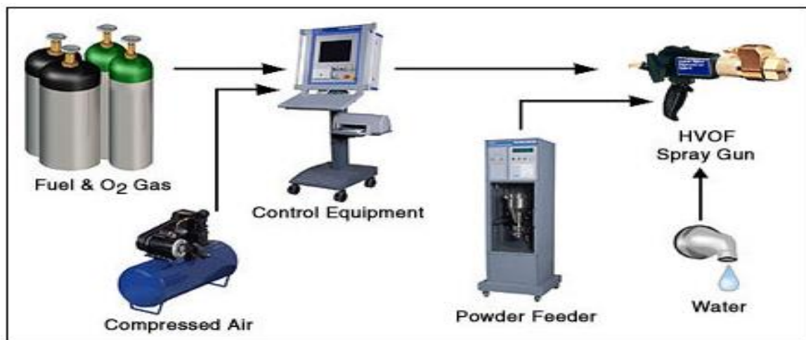
Fig.5 Key components of HVOF spray system
